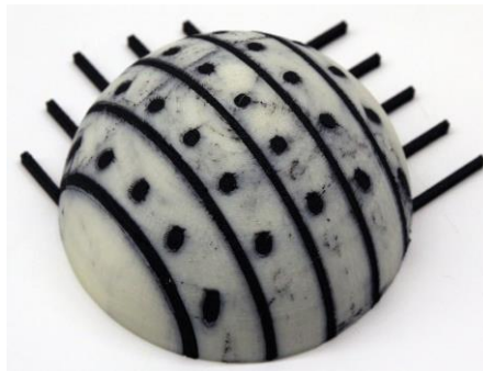
Fig. 1. X-Y Touch Pad integrated into a dome-shaped structure
