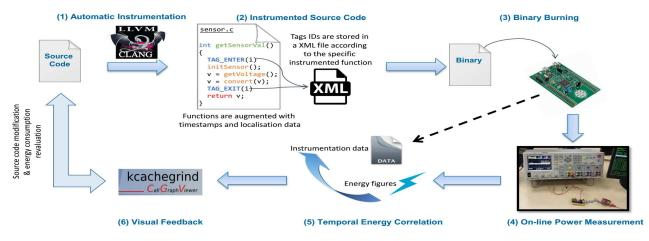
Fig. 2: The energy profiling cycle.
