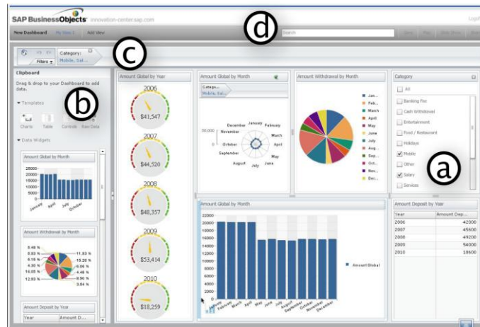
Fig 1. The Exploration Views consists of: (a) the main Dashboard and its components. (b) The Clipboard drawer widget that includes templates for charts (top) and data widget samples (bottom) that the user has created as a pallet. The drawer can be closed when not needed. (c) A visual representation of the global data filters that are active at any point. (d) And a set of other functions, such as search, save, share, etc.
