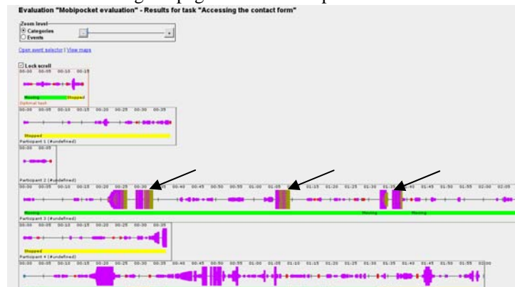
Fig. 6. Timelines referring to the access contact form. Arrows indicate mouse movements and scrolling deviation from other timelines.
