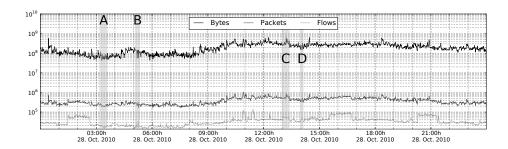
Fig. 5: Time series of three popular flow statistics; the natural and injected anomalies disappear in noise.
