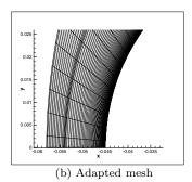
Figure 3: Comparison between a zoom of the starting nominal mesh close to the symmetry axis (left) and the same area of the adapted mesh for one of the training points (right).
