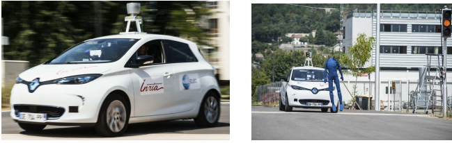
Fig. 6. Experimental Platform: Renault Zoe car equipped with Velodyne HDL64, 4 Ibeo Lux LiDARs, Xsens GPS and IMU and cameras, and a crash test dummy crossing the dedicated street for the experiments.
