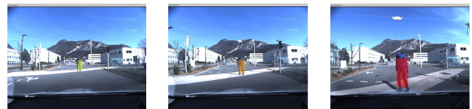
Fig. 8. Risk detection combined with automatic braking sequence. The evolution of the color of the reprojected collision risk corresponds to the time window before impact, activating accordingly the automatic braking.
