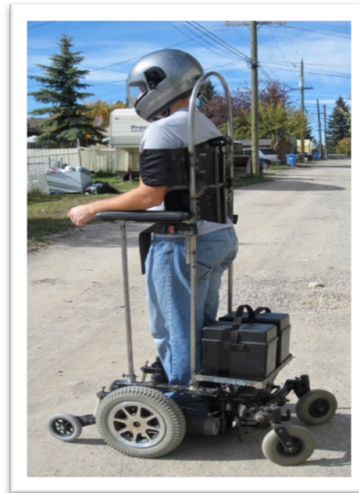
Figure 1B. Standing Platform
