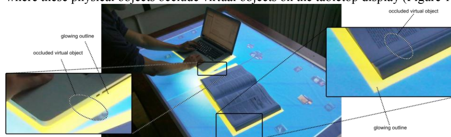
Fig. 1. Tabletop environment with physical objects (a laptop computer and a book) resting on its surface. The physical objects are occluding virtual objects on the display, so their outlines have been made to glow using one of our occlusion management techniques to indicate this.
