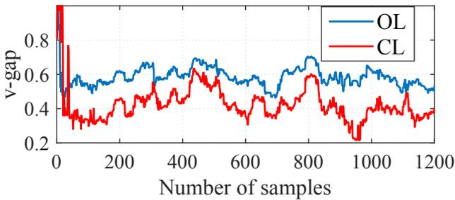
Fig. 6. CL/OL comparison through  $v$ -gap metric.
