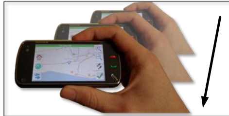
Fig.4. Zooming out using gesture zooming in IntelliTilt
