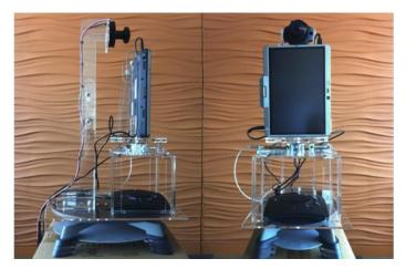
**Fig. 2.** Side and front views of the kinetic proxy. At its top is a fixed-position wide-angle video camera. Below the camera is a 12" tablet PC, which shows video of the satellite participant. The tablet is mounted atop a remotely-operated turntable which, in turn, is mounted atop a hutch that holds a videoconference speakerphone.
