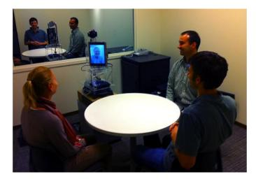
**Fig. 1.** The experimental setup, showing three collocated participants and the kinetic proxy seated around a table. The proxy was operated by a confederate, and positioned so that its swiveling display approximately matched participant eye-height.
