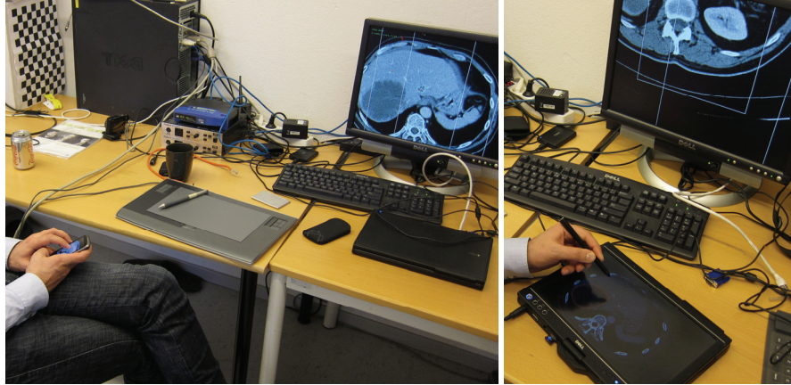
Figure 3: Surgeons and radiologists participated in interactive prototyping sessions. Left) A radiologist manipulates content on a shared display using a mobile device. Right) Interaction on a Tablet PC (Dell XT2) that supports both pen and multi-touch input.
