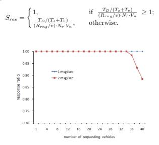
Fig. 5. Serving ratio of a responding vehicle in a target area depending on query message rate.
