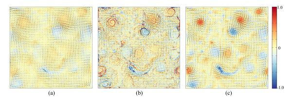
Fig. 10 Results at t = 450 on the synthetic SQG scalar image sequence: (a) estimated velocity field and vorticity map from the HS method; (b) estimated velocity field and vorticity map from Dérian et al. (2013); (c) estimated velocity field and vorticity map from the proposed method.
