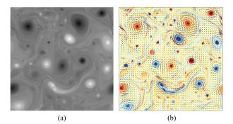
Fig. 8 Illustration of a sample frame (t = 450) from the synthetic SQG sequence: (a) passive scalar image; (b) the simulated ground-truth velocity field with vorticity map, which is used for evaluation of the estimated motion hereafter.
