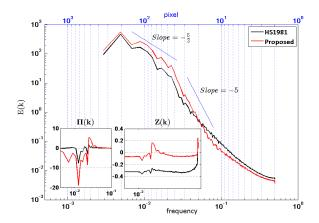
Fig. 13 Spectrum analysis of the turbulent velocity for experimental scalar images. E(k) denotes the energy at a given frequency,  $\Pi(k)$  and Z(k) the energy flux and enstrophy flux, respectively.
