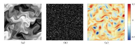
Fig. 1 Illustration of a sample frame (t = 50) from the DNS synthetic image sequence: (a) passive scalar image; (b) particle image; (c) vorticity map with the ground-truth velocity field.
