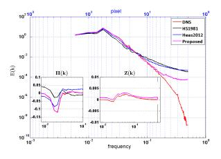
**Fig. 5** Spectrum analysis of the turbulent velocity for DNS scalar image sequence. E(k) denotes the energy at a given frequency,  $\Pi(k)$  and Z(k) the energy flux and enstrophy flux, respectively. For clarity reasons the enstrophy fluxes of Héas et al. (2012) and HS method are not shown. They are almost constant with a value of 0.17 and -0.08 for Héas et al. (2012) and HS method, respectively.
