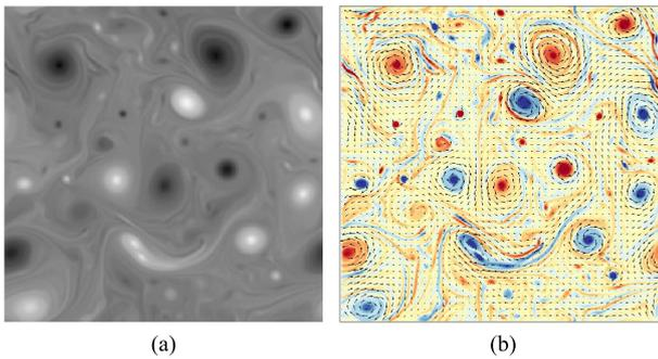
**Fig. 8** Illustration of a sample frame ( $t = 450$ ) from the synthetic SQG sequence: (a) passive scalar image; (b) the simulated ground-truth velocity field with vorticity map, which is used for evaluation of the estimated motion hereafter.
