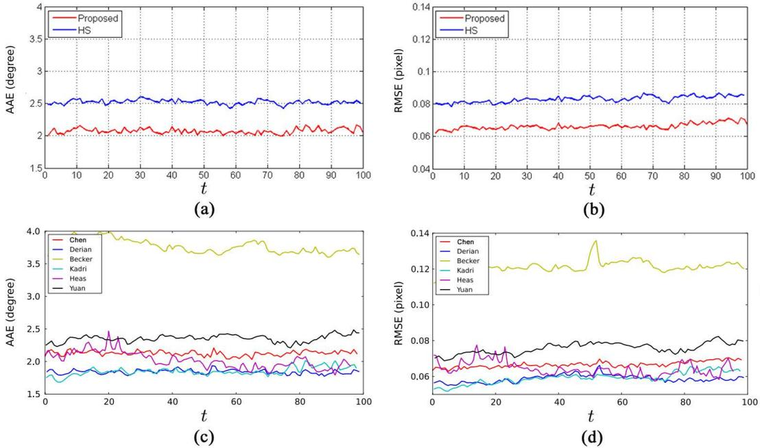
**Fig. 6** AAE (left) and RMSE (right) errors of different estimators for DNS particle image sequence. Results of the proposed method are plotted in figures (a) and (b), in comparison with the results of the HS method. The data of several state-of-the-art approaches, shown in figures (c) and (d), are extracted from Chen et al. (2015).
