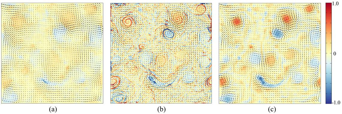
Fig. 10 Results at  $t = 450$  on the synthetic SQG scalar image sequence: (a) estimated velocity field and vorticity map from the HS method; (b) estimated velocity field and vorticity map from Dérian et al. (2013); (c) estimated velocity field and vorticity map from the proposed method.
