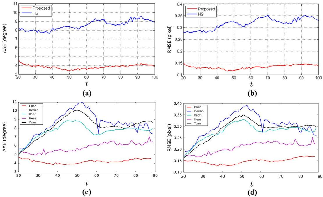
**Fig. 4** AAE (left) and RMSE (right) errors of different estimators for DNS scalar image sequence. Results of the proposed method are plotted in figures (a) and (b), in comparison with the results of the HS method. The data of several state-of-the-art approaches, shown in figures (c) and (d), are extracted from Chen et al. (2015).
