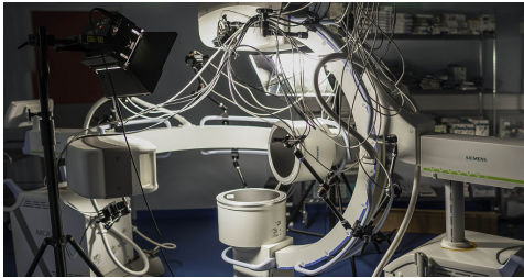
Figure 7: Proposed capture platform actual implementation: X-ray amplifiers and 10 video cameras surrounding the acquisition volume. Note that only a single amplifier is actually used in the proposed approach.
