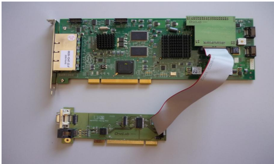
Fig. 2. Printed board composing the core of the probe for timestamping through Global Positioning System (GPS)
