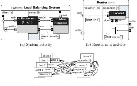
(c) Structural view of system example with four clients and two servers
