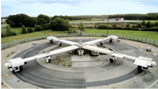
**Fig. 1** Accelerated pavement testing facility of IFSTTAR.
