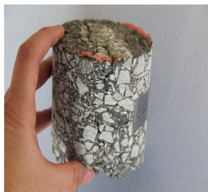
**Fig. 12** Photograph of the cores taken from the HMAM structure.
