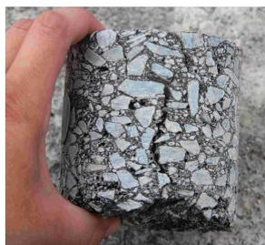
**Fig. 13** Photograph of the cores taken from the DGBM structure.
