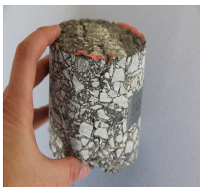
Fig. 12 Photograph of the cores taken from the HMAM structure.
