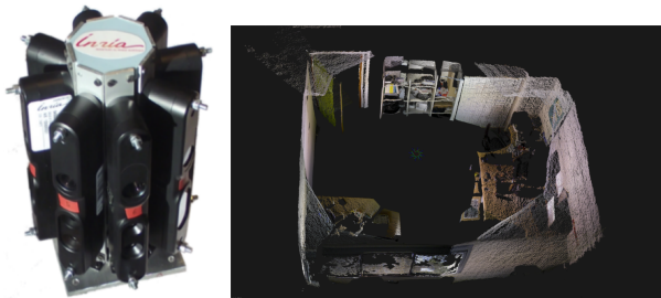
Fig. 4. Omnidirectional RGB-D acquisition device with 8 Asus Xtion Pro Live (Asus XPL) sensors mounted vertically in a radial configuration (left plot) and respective point cloud of one of the offices used in the real sequence (right plot).
