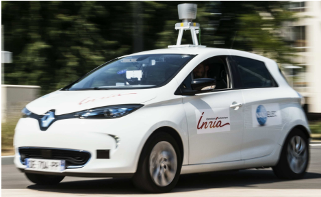
Fig. 4. Experimental Platform: Renault Zoe car equipped with Velodyne HDL64, 4 Ibeo Lux LiDARs, Xsens GPS and IMU and cameras.
