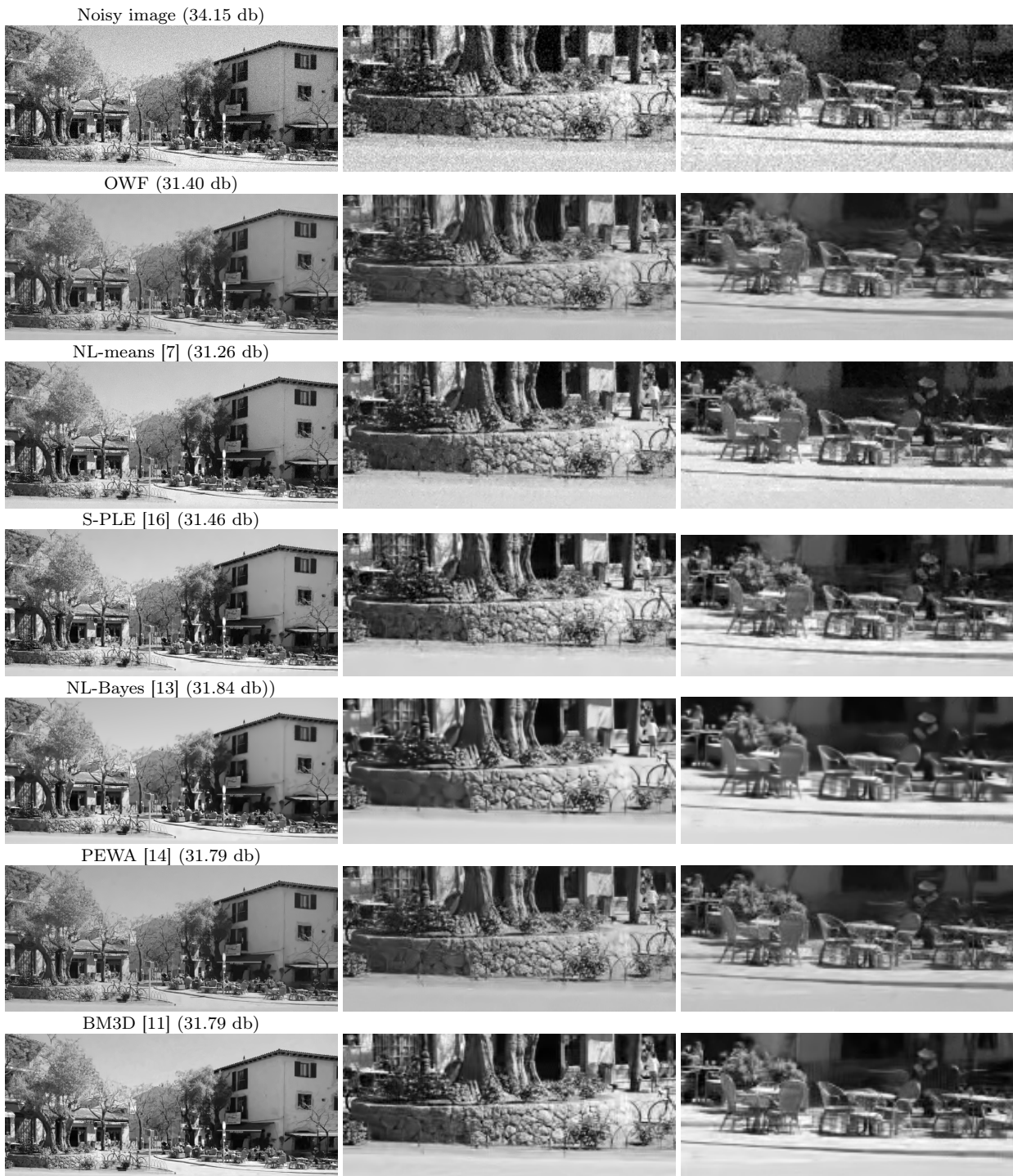
FIGURE 8 – Comparative results on the “valldemossa” image corrupted with WGN ( \sigma = 15 ). From top to bottom : noisy image, OWF, NL-means [7], S-PLE [16], NL-Bayes [13], PEWA [14], BM3D [11].
