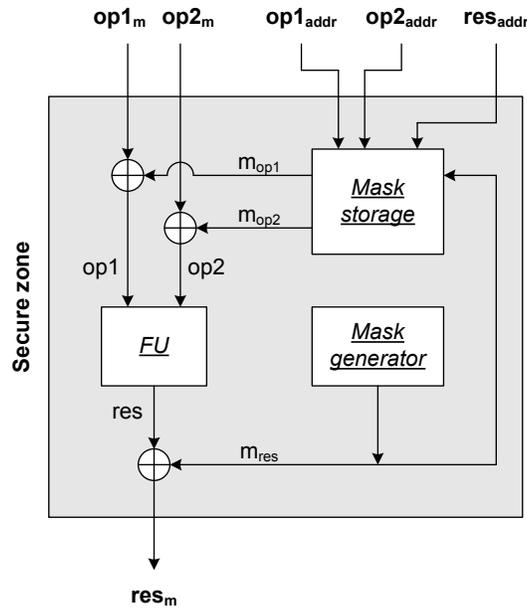
**Fig. 2.** The secure zone of the Power-Trust platform.
