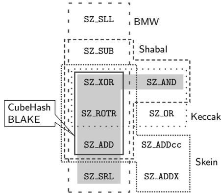
**Fig. 3.** Generic commands required from the secure zone to implement SHA-3 candidates. With the exception of `SZ_R0TR` they have an unprotected equivalent in the SPARC V8 instructions (see appendix B, [31]).
