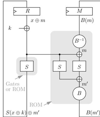
Fig. 4. Mask path with bijections for “Leakage squeezing”.
