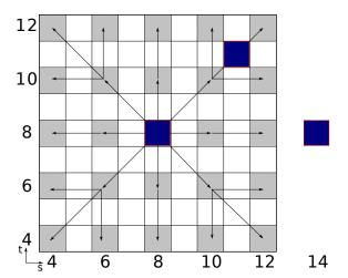
Figure 7. Light field setup for experiments. Cameras from the Stanford dataset are arranged on the same plane (s, t). Each cell is a view from the original dateset. Grey cells are views that are used to sample the plenoptic space. Arrows indicate how the optical flow is performed. Blue cells are view we synthesize to evaluate our method. We interpolate views (8, 8) and (11, 11), and extrapolate view (14, 8).
