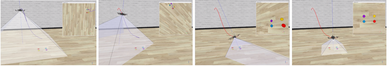
Fig. 4. Successive snapshots taken from V-Rep at different time instants. The straight line represents the vertical axis of the camera, the blue line is the planned trajectory and the red line is the actual system trajectory. The camera view is shown in the upper right corner.
