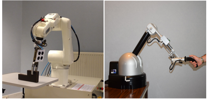
Fig. 1. Left: the slave manipulator arm. The object to be manipulated is on the table in front of the slave robot. Right: The master device used by the operator for sending commands to the slave manipulator and receiving force cues.
