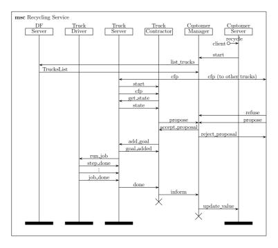
Fig. 1. Agent processes and message exchange in EcoTruck
