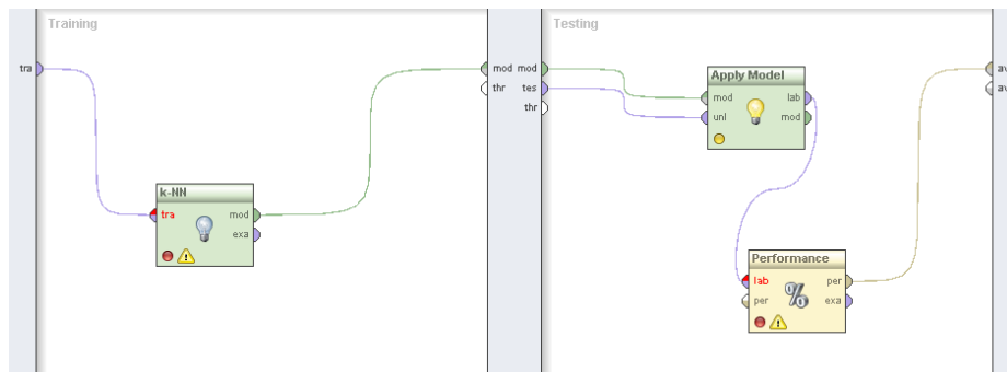
Fig. 2. The embedded training and testing process for a k -nn classification model in Rapidminer workflow.
