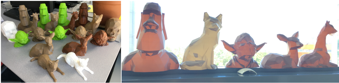
Figure 6: The models used for comparing with the work of Lee et al. [15]. Right . Printing without inner shell makes the models transparent enough to let us see the inner cavities.
