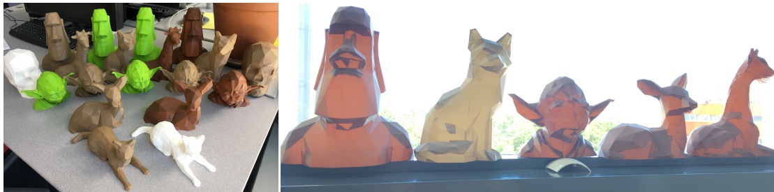
Figure 7: The models used for comparing with the work of Lee et al. [17]. Right . Printing without inner shell makes the models transparent enough to let us see the inner cavities.
