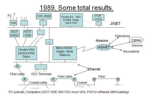
Figure 5. Use of Ethernet connections at the end of the 1980s.
