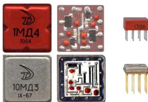
Figure 7. First series IC in the USSR, “Tropa”, thick-film, a top number, “Posol”, thin-film, the bottom number. (At the left and in the center – in the double size, on the right – in full size).
