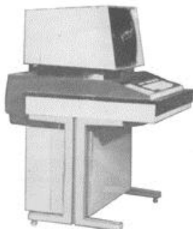
Figure 2. The device of visual display (UVO). The symbolical display. Diagonal of the screen (43 cm); Size of the screen (220x200 mm); Symbols (up to 2048); Lines on the screen (32); Symbols in line (64); Size of a symbol (3.5x2.5 mm); Ensemble of symbols (128).
