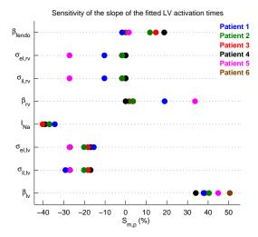
**Figure 5** Significant parameters following sensitivity analysis results for the slope of the fitted line between simulated and measured activation times for the six patients (different colors for each patient).
