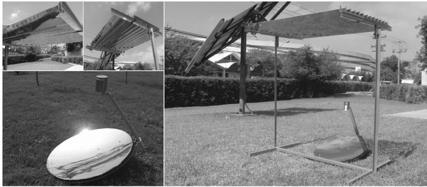
Fig. 9. Semi-passive solar concentrator prototype
