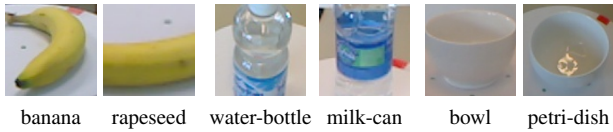
Fig. 9: Object labels for different sample patches using a pre-trained CNN ( AlexNet ). It often fails when patches contain only partial views of objects (banana and water bottle) or unexpected points of view (bowl).
