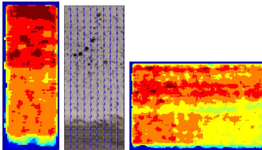
**Fig. 6.** Representation of displacement map (left) where the dark regions indicated larger displacements, the vector diagram (centre) shows the flow of deformation and with the same system is also possible to compute the complete displacement map (right).
