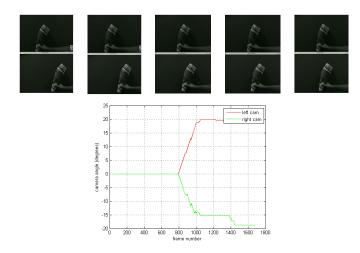
**Fig. 4** – Real-time image alignment process frame sequence (each colum pair is an stereo pair). Below are the left camera angle values (red line) and right camera angle values (green) in degrees during the image alignment process.
