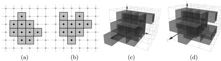
**Fig. 1.** Convexity alterations under rotation: (a) a convex digital object in 2D, and (b) its non-convex transformed image by a rotation; (c) a convex digital object in 3D, and (d) its non-convex transformed image by a rotation.
