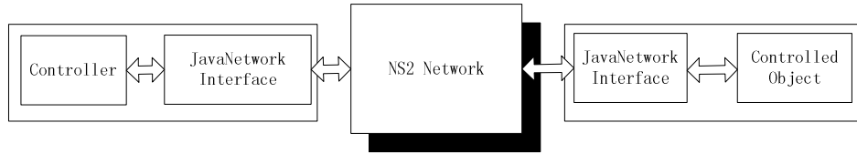
Fig.3 the framework of testing bed based on NS2
