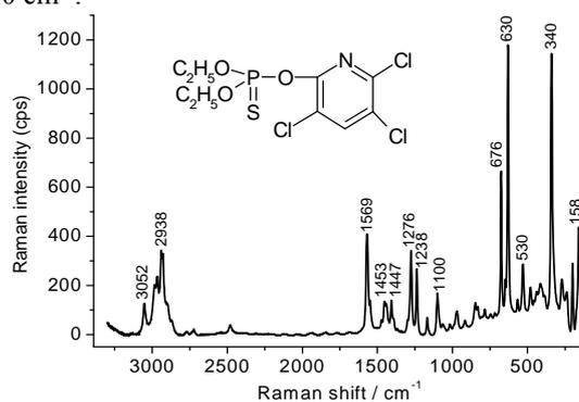
**Fig. 2.** Raman spectrum and molecular structure of chlorpyrifos.
