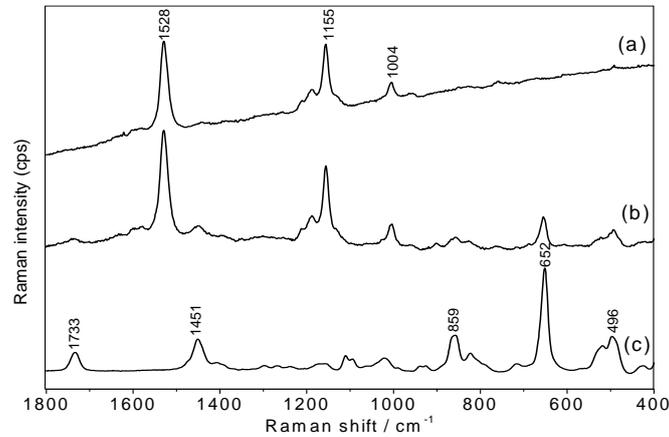
**Fig. 6.** Raman spectra of (a) orange's pericarp, (b) malathion formulation (40% w/w) left on the surface of orange and (c) standard malathion solution.
