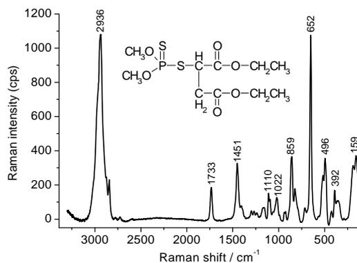
**Fig. 4.** Raman spectrum and molecular structure of malathion.
