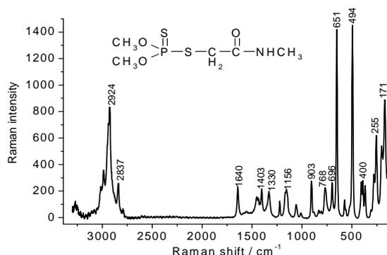
**Fig. 3.** Raman spectrum and molecular structure of dimethoate.
