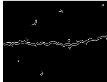
Fig. 16. Result of canny edge detection.
