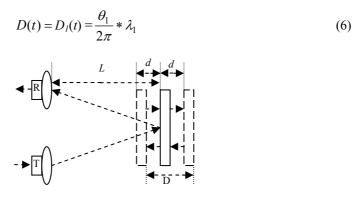
Fig.1. Schematic diagram of ultrasonic system for vibration measurements.
