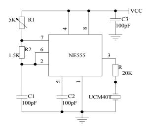
Fig. 3. the circuit for ultrasonic transmitting.
