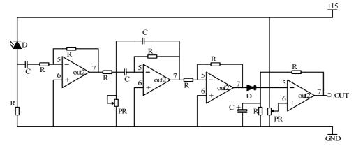
Fig.4. the circuit for ultrasonic receiving.
