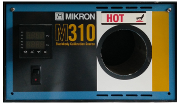
(a) Mikron M310 blackbody calibration source
