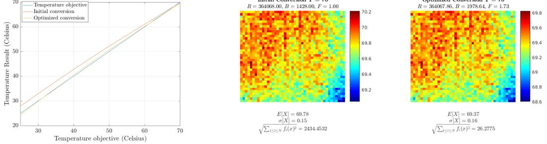
(a) Calibration optimization result (b) Calibration differences example at 70°C
