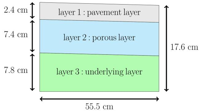
Figure 2: Sectional schematic view of modified road structure
