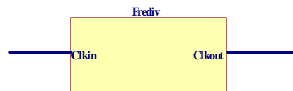
Figure 9 Logic Diagram of Baud-rate Generator
